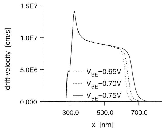
Fig. 8 Electron drift velocity for  $V_{CB} = 2.0$  V.
