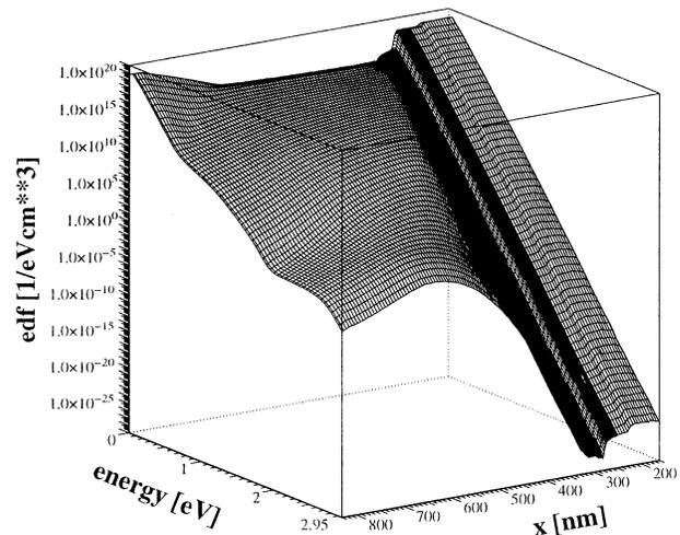
Fig. 11 Electron energy distribution function for  $V_{CB} = 2.0$  V and  $V_{BE} = 0.75$  V.
