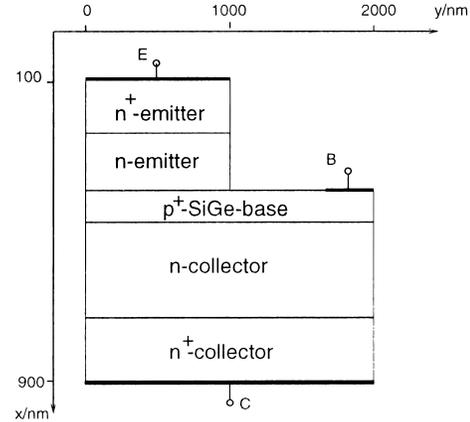
**Fig. 4** The 2D SiGe-HBT test structure.
