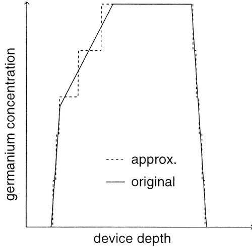
**Fig. 1** Original germanium profile and approximation for the selection of the band structures.
