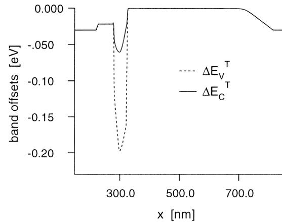
**Fig. 5** Conduction and valence band offsets.
