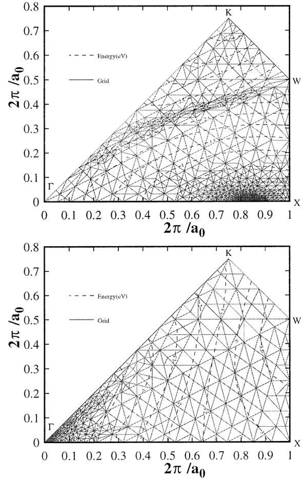
**Fig. 2** Nonuniform adaptive tetrahedral mesh of the first conduction band (upper graph) and of the first valence band (lower graph) in the  $k_x, k_y$ -plane. Equienergy lines are for relaxed Si.
