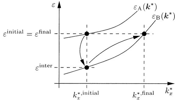
**Fig. 3** Selection of the final state after a heterointerface transition from band structure A to B.
