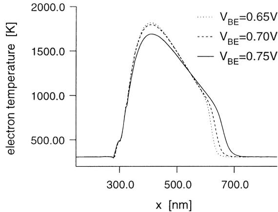
Fig. 9 Dynamic electron temperature for  $V_{CB} = 2.0$  V.
