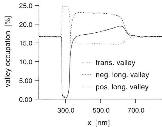
Fig. 10 Relative electron population for  $V_{CB} = 2.0$  V and  $V_{BE} = 0.70$  V for a transversal valley, the negative and positive longitudinal valley.
