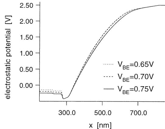
Fig. 6 Electrostatic potential for  $V_{CB} = 2.0$  V.
